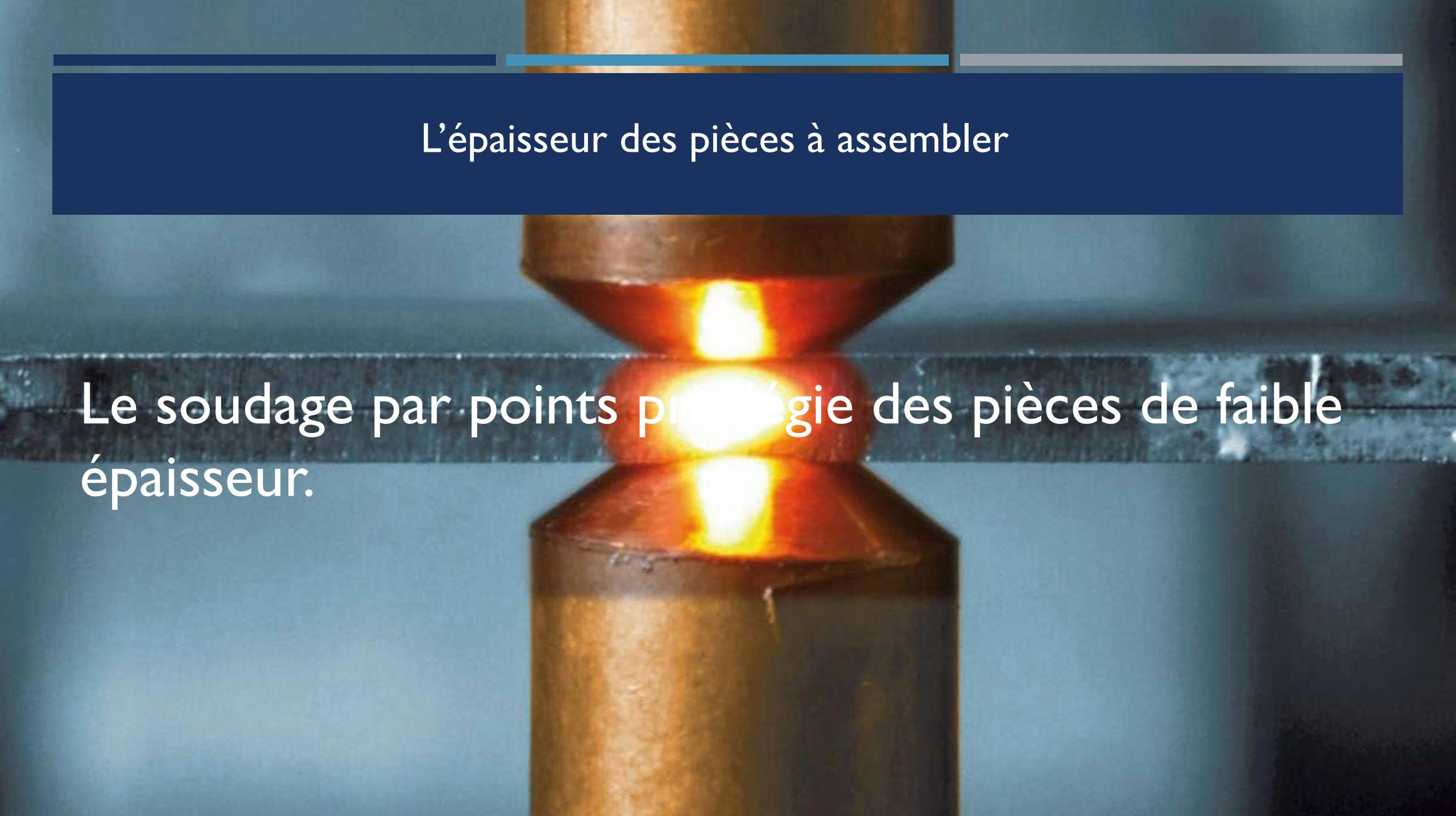
A close-up photograph of a resistance spot welding process. Two copper-colored cylindrical electrodes are positioned vertically, clamping a thin metal plate between them. At the point of contact, a bright yellow-orange glow indicates the heat generated by the electrical current. The background is a dark, industrial setting.
